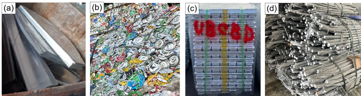
Fig.1. (a) new scraps, (b) UBC bale, (c) RSI-A, and (d) aluminum cable wires.
